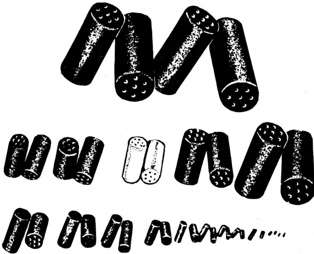
Figure 10-3. — Smokeless powder grains.
